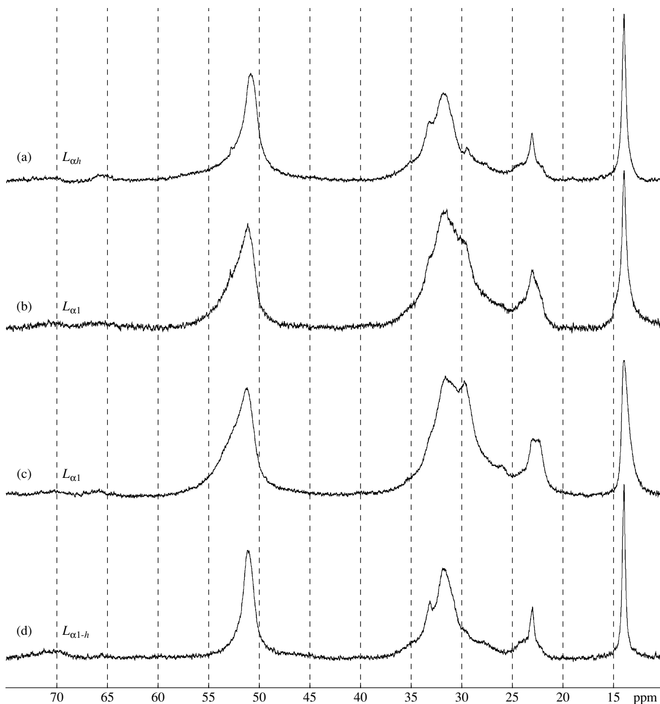
Fig. 3. The ^{13}\text{C} NMR spectra from the (a) L_{\alpha h} , (b, c) L_{\alpha l} , and (d) L_{\alpha l-h} phases. The spectrum of the L_{\alpha l} phase indicates the formation of two phases on cooling from the temperature of the isotropic state (360 K) to initial room temperature (295 K).
